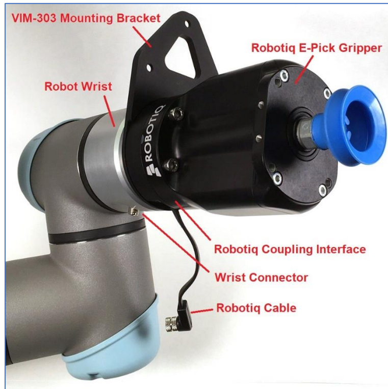
Figure A14 - Attaching the Robotiq E-Pick Gripper
