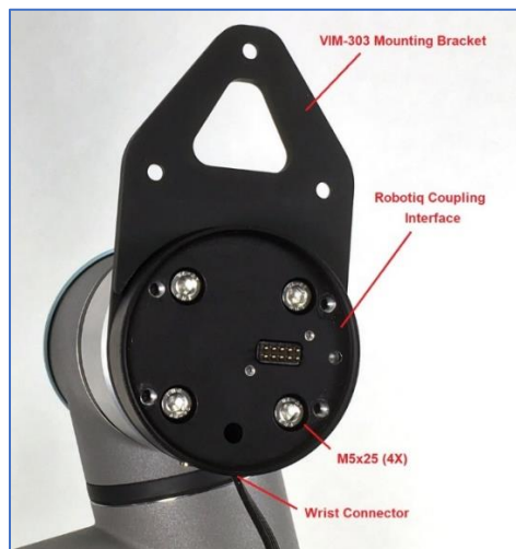
Figure A20 - Attaching VIM-303 Mounting Bracket and Robotiq Coupling Interface
