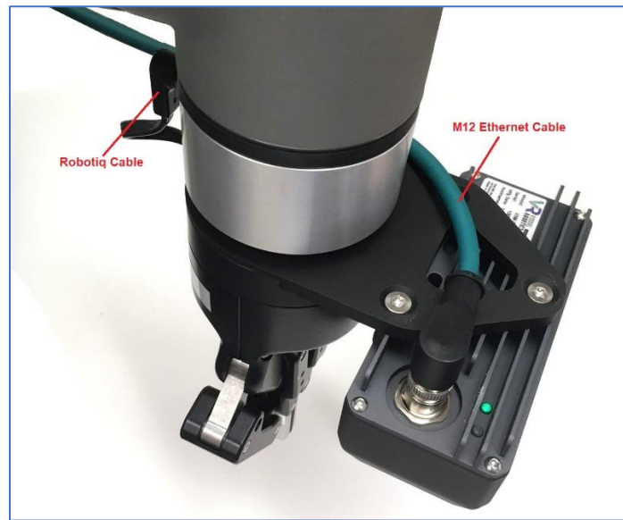
Figure A23 - Attaching Cables
