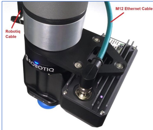
Figure A16 - Attaching Cables
