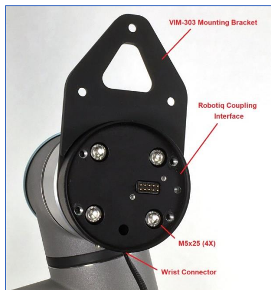
Figure A13 - Attaching VIM-303 Mounting Bracket and Robotiq Coupling Interface
